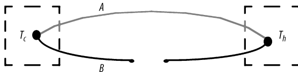
Figure 9.1. Thermocouple basic circuit
